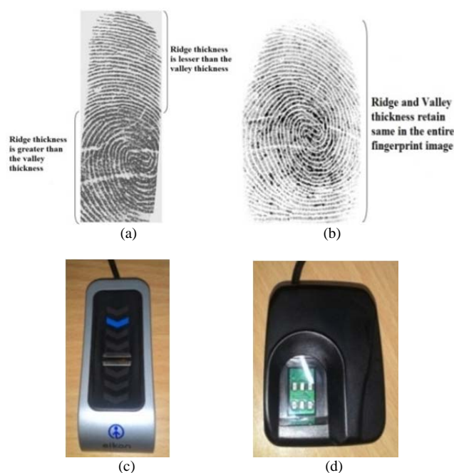
Fig. 1(A) Image Captured By Capacitive (Swipe) Sensor Shown In (C) and (B) Image Captured By Optical (Press or Thumb) Sensor Shown In (D)
